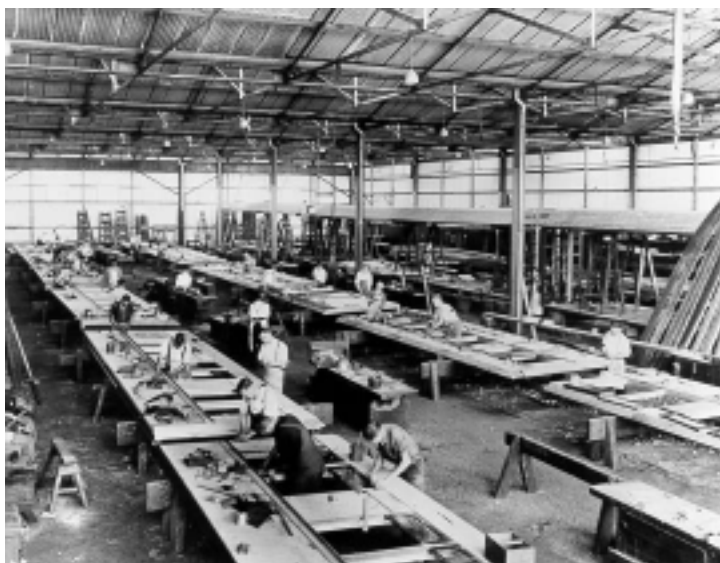
Figure 3.119: Converting 'box' or 'express' cars to corridor type cars in the Carriage Shops Extension (now called the Cable Store) probably in the 1930s. Source: SRAO.
